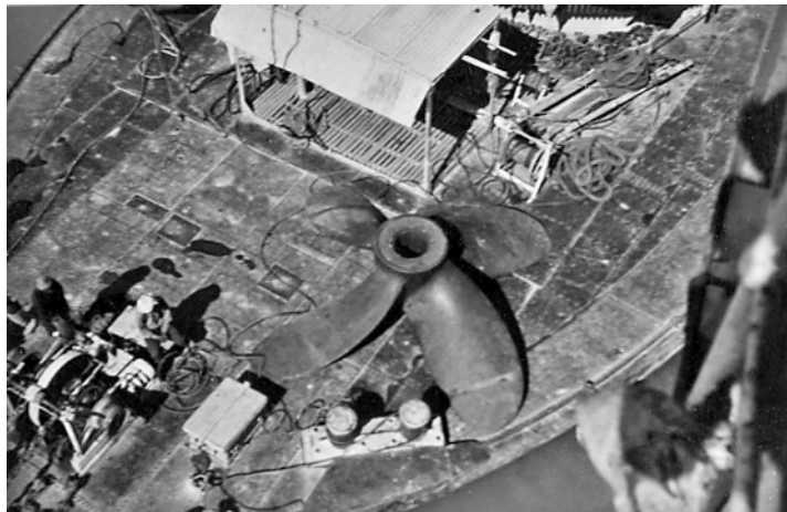
The spare propeller lowered onto the barge, ready for fitting
