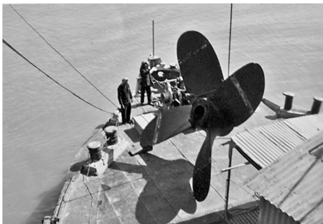
The spare propeller lowered onto the barge, ready for fitting
