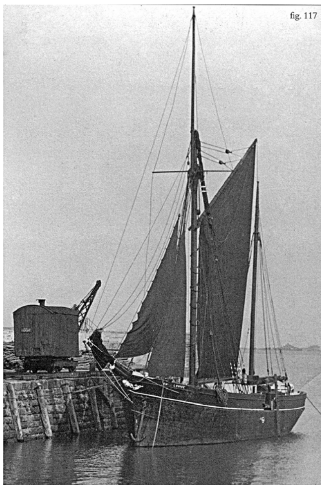
The photograph shows the "Emma Louise" alongside in Minehead harbour with her sails up to dry before loading pit props seen on the quay beside her, and was taken in 1932. This is before her conversion to an auxiliary sailer and so she still carries a jib boom, topmast and full suit of sails. The steam crane is alongside her, and must have been nearly as old as the ship.
