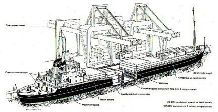
These 4000 ton cellular container ships, which could load 148 boxes, were the first to be built in Britain, at John Readheads, South Shields, in 1967/8. They were withdrawn from service in '86 and Sea Freightliner 2 was broken up at Gadani Beach in 1987.
