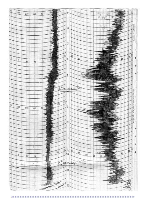
Above, the wind speed and direction as recorded at Southampton Port Radio (now VTS). The maximum recorded was 83 knots shortly after 0300 but I believe more than a hundred was showing at Fawley at that time.
