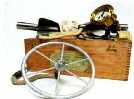
The Walker's "Cherub III" Taffrail Ship-Log
